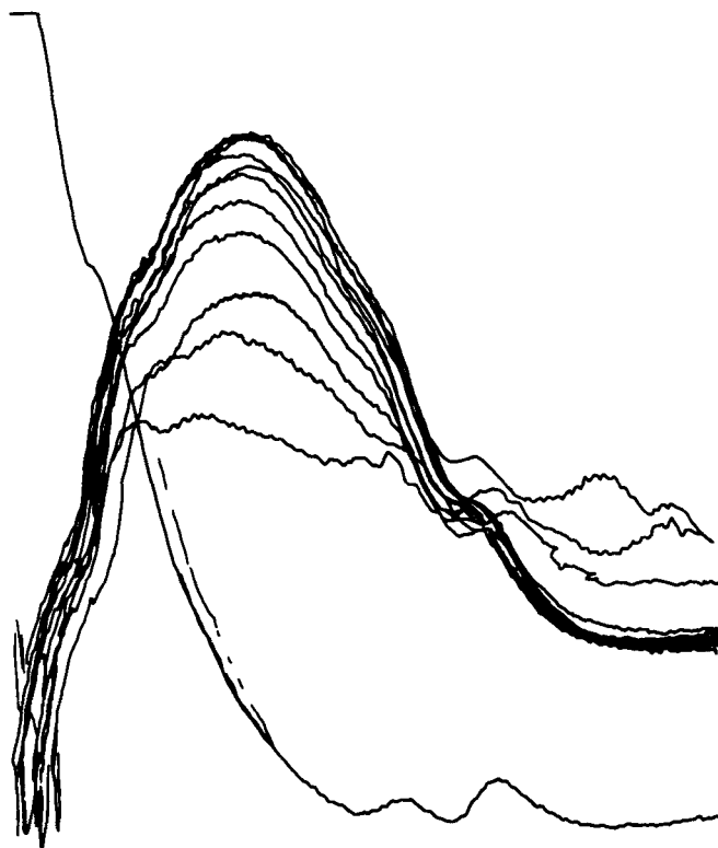
FIGURE 5 Repetitive scan spectrum between 363 and 550 nm (from left to right) that results on addition to a mixture of 0.7 ml "solvent" (contains 0.1 M pyrophosphate, 1 mM TDP, 1 mM \text{MgSO}_4 , 0.5 mM EDTA, 0.5 mM phenylmethane sulfonyl fluoride) and 0.2 ml of 10 mM m -NPB (in both reference and sample cuvettes), 200 \mu\text{l} (160 units/ml or about 30 units total) PDC in the sample cuvette only at 10°C. The spectra were recorded at 0.1 absorbance range, 3 nm band width, 2 nm/s and 10 nm/cm in a 1 ml 10 mm path cuvette. The maximum is near 430 nm.
